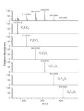
Direct liquid measurement for determination of OMEs in biofuels.
