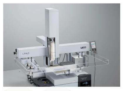
All L-PAL3 models are CTC-based robots that combine an autosampler and an injector that operates in three dimensions of space.
