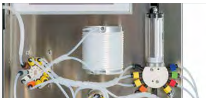
Automated sample loading
