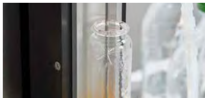
Rinsing of sample vial for quantitative transfer
