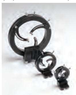
Fig. 1 Cylindrical Sample Holders for D25 mm, D50 mm, and D110 mm Respectively (in order from front to back)
