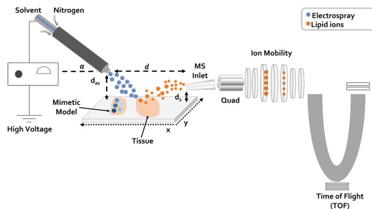
Figure 1. Schematic representation of desorption electrospray ionization (DESI) mass spectrometry imaging ion source coupled with quadrupole time-of-flight (ToF) mass spectrometer equipped with ion mobility separation
