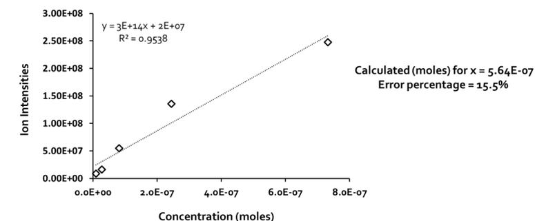
Figure 5. The peak intensity of ROI corresponding each concentration was exported as an individual mass spectrum. The ion intensities of analyte standard for each plot was plotted and fitted with linear trendline. Based on the equation, unknown concentration for X was calculated. The error was calculated based on real known concentration of the X.
