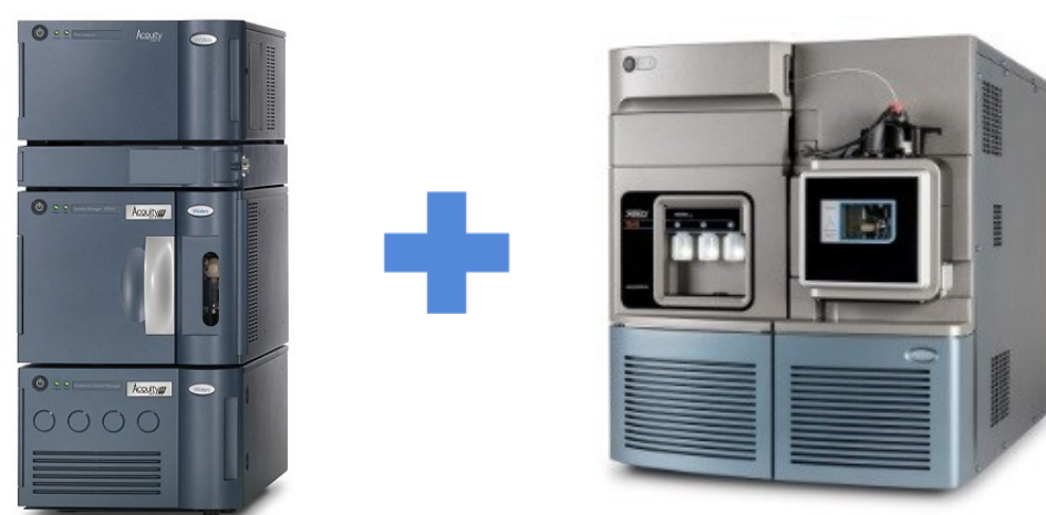
Figure 1. Waters ACQUITY UPLC H-Class coupled to the Xevo TQXS tandem mass spectrometer
