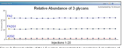
Figure 2: Reproducibility of the LC system demonstrated by monitoring 3 glycoforms of varying relative abundances over 20 consecutive injections. Sample was Waters' RFMS glycan standard. Relative abundance was calculated based on the ratio of area for selected peaks vs the total calculated peak area for all glycoforms.
