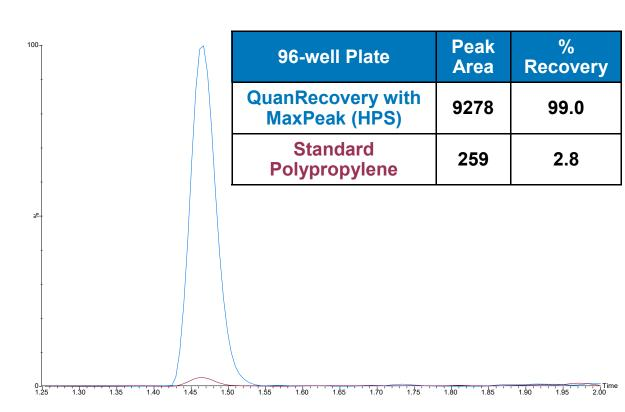
Figure 2. Peak area and recovery of 10 ng/mL pramlintide stored in standard polypropylene and QuanRecovery with MaxPeak (HPS) 96-well plates.
