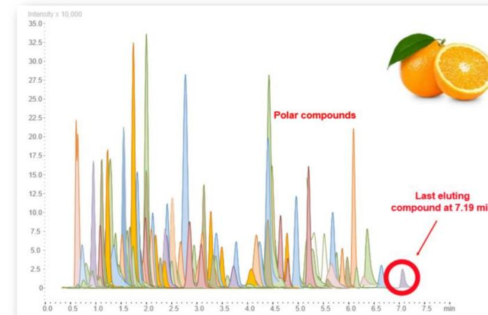
Figure 2: 164 pesticides spiked at the default MRL of 0.01 mg/kg (orange matrix). Quantifier ion is shown
