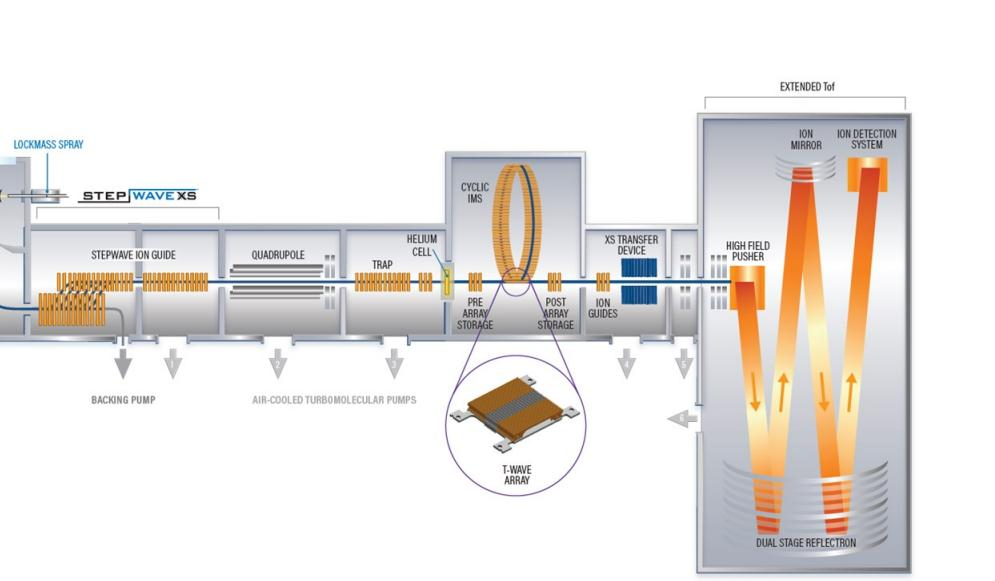
Figure 1. Schematic of the cIM device embedded in a Q-cIM-ToF geometry.
