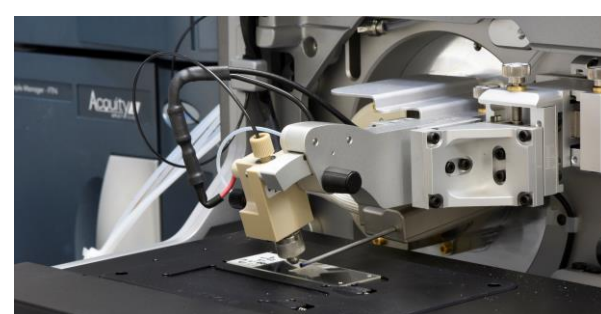
Figure 2. DESI XS ion source mounted on Waters Xevo TQ Absolute mass spectrometer.
