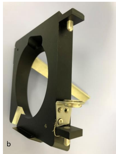
Figure 10: iButton on original ESI Source (a); iButton on the SICRIT Interlock (b).
