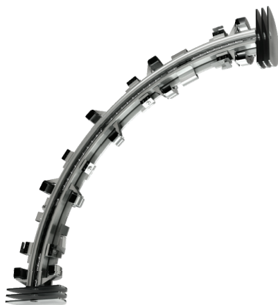
FIGURE 2. Q2 from the TSQ Quantiva MS. Fragment ions are accelerated through the cell with the application of an axial DC potential, enabling data acquisition at dwell times as low as 1msec without signal loss. This facilitates the ability to acquire in excess of 500 SRMs/second.
