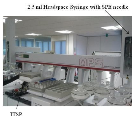
Figure 3: Detail photograph for automated SPE
