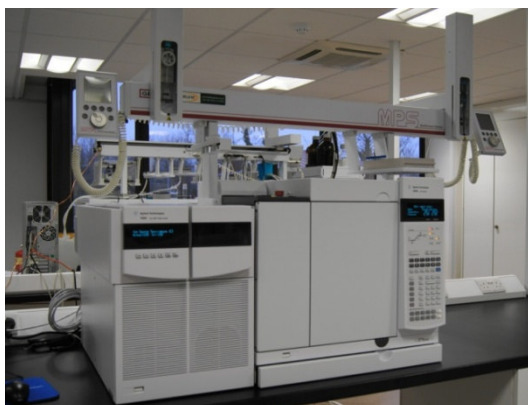
Figure 2: Gerstel Dual Head MPS with GC/MS/MS Triple Quadrupole
