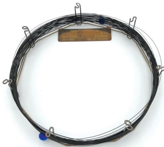
Figure 7B. An Agilent J&W DB-5ht after operating at 400 °C for 25 hours.
