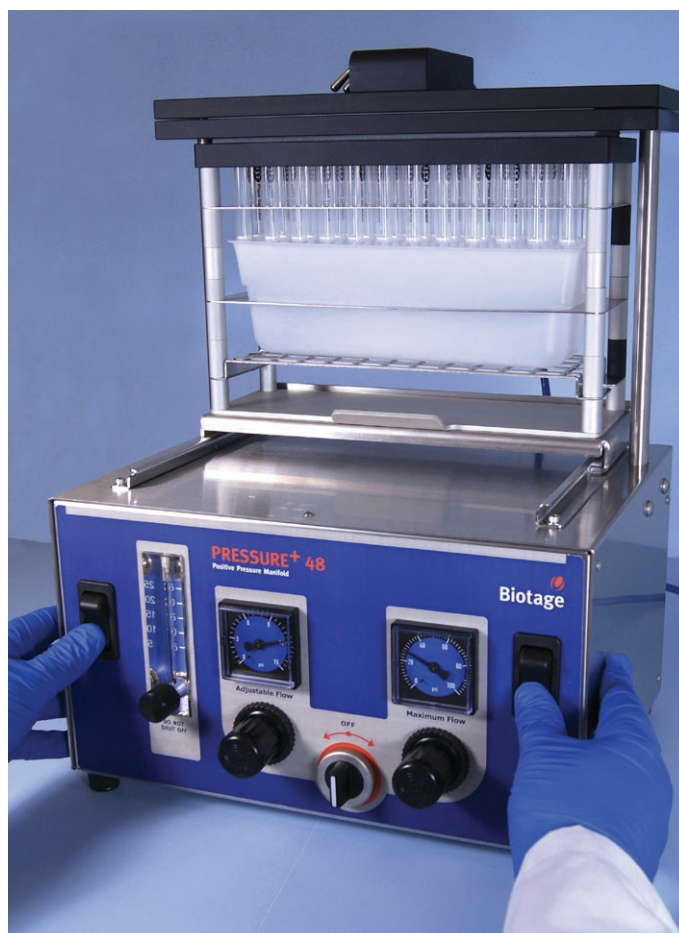
Figure 2. Lower the manifold by pressing down on the two rocker switches simultaneously for approximately 3 seconds.
