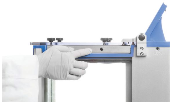
Figure 7. If using a TurboVap II rack without end-point sensors, a manifold air shield has to be installed.
