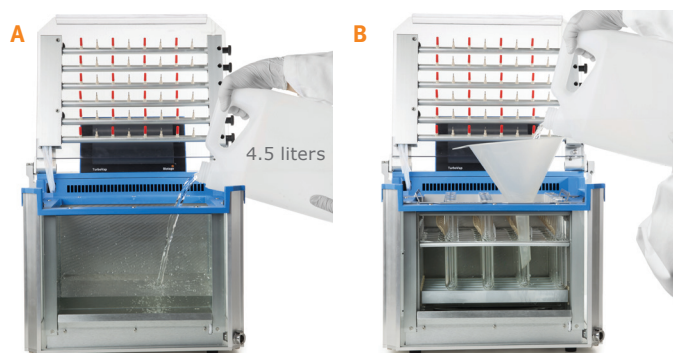
Figure 2. The water's surface must be above the minimum level marked on the water bath but not higher than just below the blue water bath top cover.
