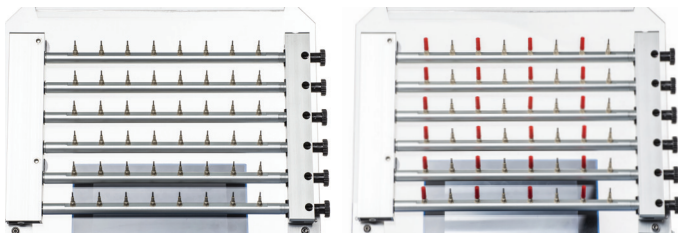
Figure 14. TurboVap LV manifold with 48 nozzles (left). In the picture to the right, 24 nozzles are plugged for usage with the multi rack with 24 positions.
