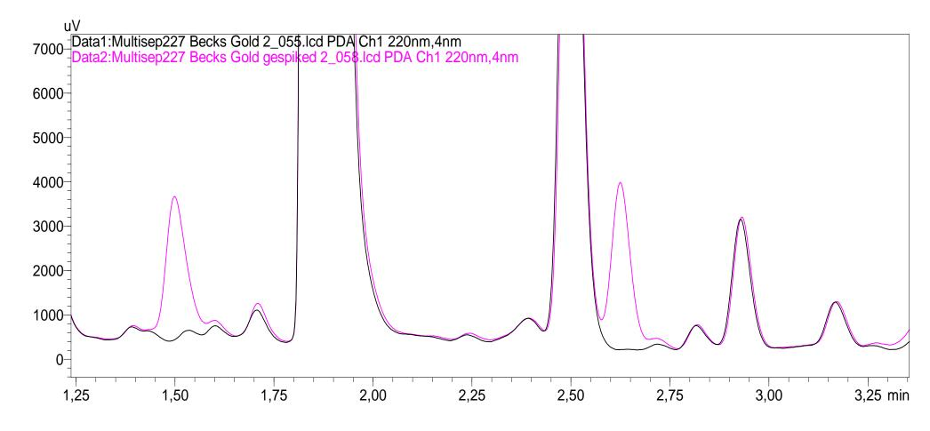
Figure 3: PDA Chromatogram of spiked and non-spiked beer sample
