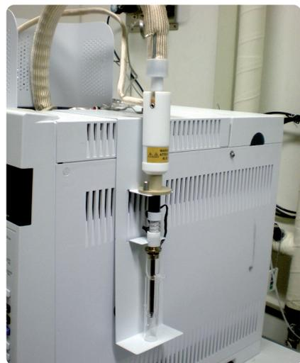
**Figure 2.** Docking station for GC-ICP-MS interface kit located on the right hand side of the GC
