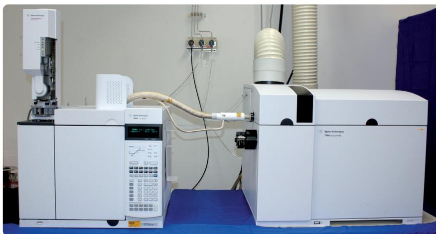
**Figure 1.** New GC-ICP-MS interface kit (G3158C) connected to an Agilent 7700 Series ICP-MS
