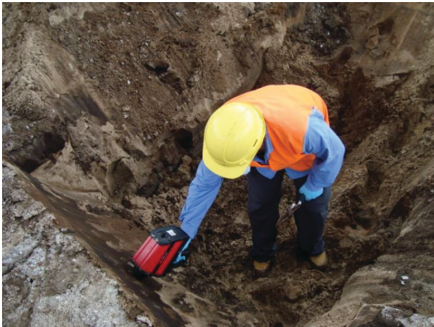
Figure 1. Agilent FTIR analyzer with diffuse reflectance sampling interface rapidly records the molecular spectrum of the sample with no preparation required
