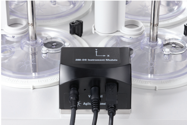
The 280-DS Instrument Module positioned on the vessel plate to measure level (X and Y axes) and vibration (X, Y and Z axes).
