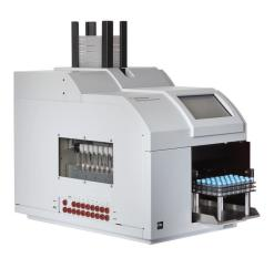
The Agilent 850-DS automates the process of dissolution sample transfer, filtration and collection. This integrated workflow solution provides for unattended sampling to increase reproducibility and free up analyst time.
