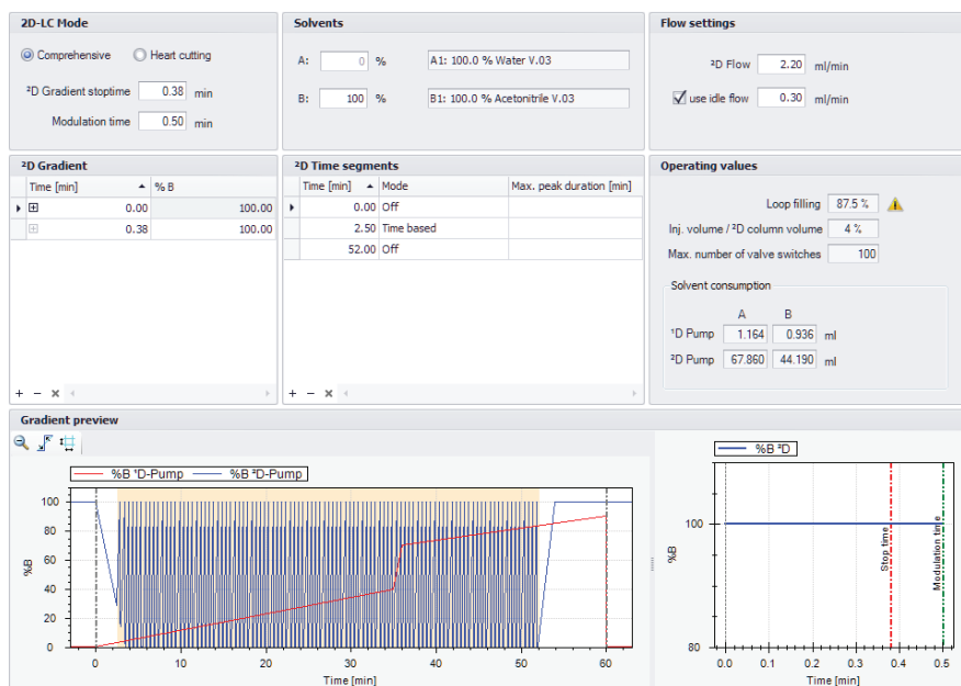
Figure 2. Screenshot of the 2D-LC method (OpenLAB CDS ChemStation)
