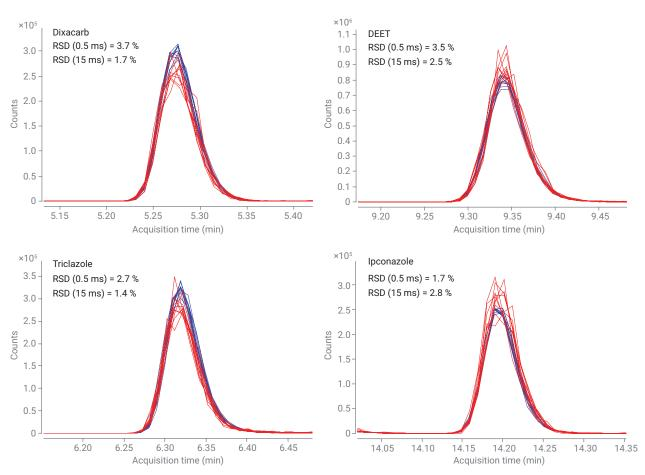
A comparison of an analysis for various pesticides acquired at 15 ms and 0.5 ms dwell times (20 pg on-column).
