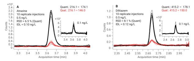
Overlaid MRM chromatograms for two example PPCPs evaluated in this study at 0.5 ng/L. Reproducible responses (RSD% <10 %) were observed for both quantifier and qualifier ions of atrazine (A) and diltiazem (B) at sub-ng/L concentrations.
