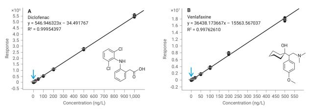
Calibration plots for diclofenac (negative mode) and venlafaxine (positive mode) in water evaluated for quantitation accuracy and peak area RSD.
