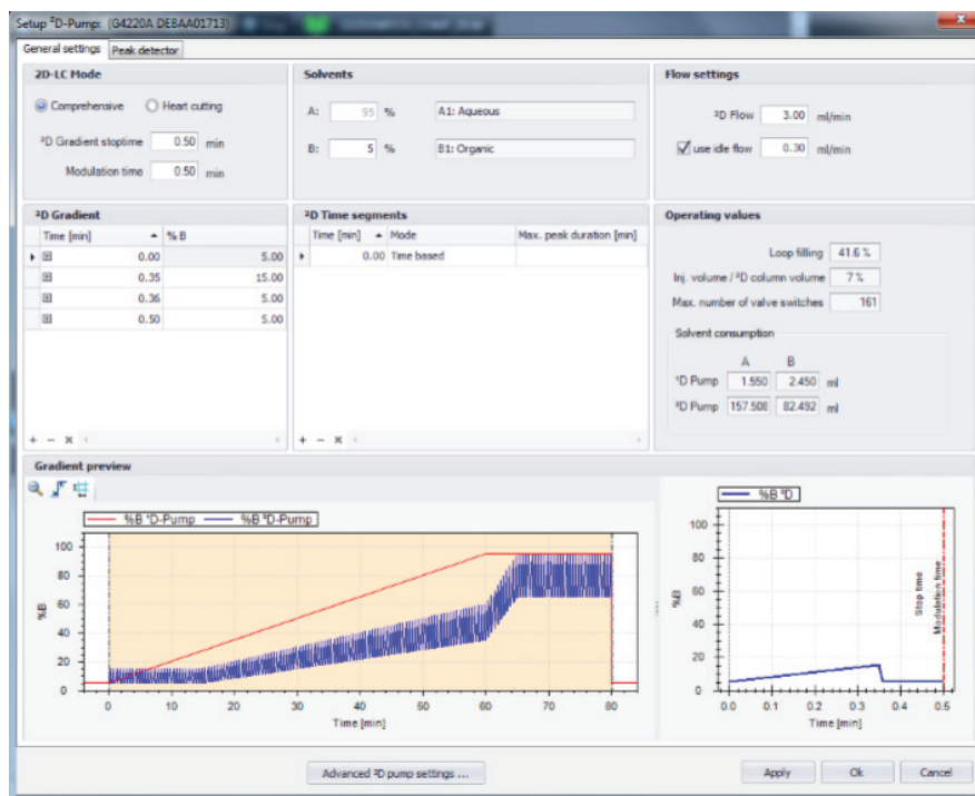
Figure 4. Method setup for the second dimension pump.
