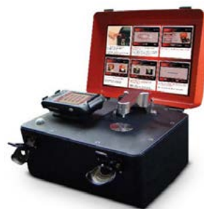
Figure 1. Agilent 4500 Series FTIR, a battery powered, portable FTIR, equipped with 100- \mu\text{m} pathlength TumbllIR sample interface for the measurement of ^2\text{H}_2\text{O} .
