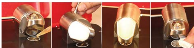
Figure 2. TumbIR operation: Place sample on window; rotate second window into position; analyze sample; clean windows by wiping.
