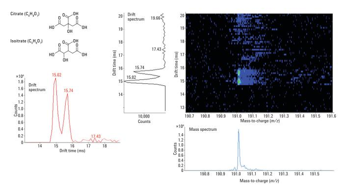
Citrate and isocitrate are isomers that are very similar in physical properties and structure. This presents challenges in their bio-analytical characterization. The Agilent 6560 Ion Mobility Q-TOF LC/MS shows clear resolution between these isomers.
