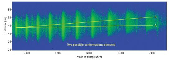
Two protein conformations are detected in the native IgG-1 sample using the 6560 system.
