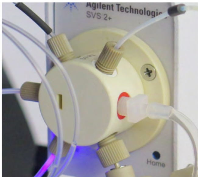
Figure 2. Agilent SVS 2+ Switching Valve System showing the 7 port switching valve (6 ports plus a slot for a T-connector).
