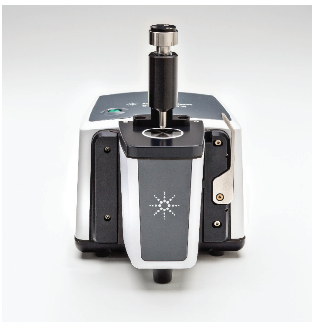
Figure 1. Agilent Cary 630 FTIR instrument with ATR sampling accessory attached.
