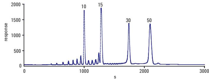
High resolution separation of a poly-T-oligonucleotide size standard spiked with 10, 15, 30 and 50 mer (main peaks).
