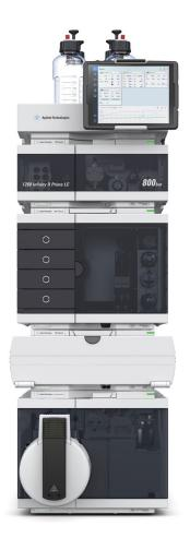
Agilent Ultivo Triple Quadrupole LC/MS and 1260 Infinity II Prime LC
