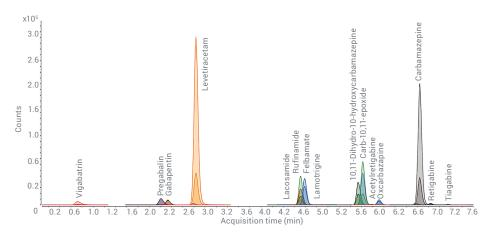
Overlays of (15) Dynamic MRM (dMRM) chromatograms of antiepileptic drugs in human serum achieved under 8.0 minutes on the Ultivo LC/TQ system.
