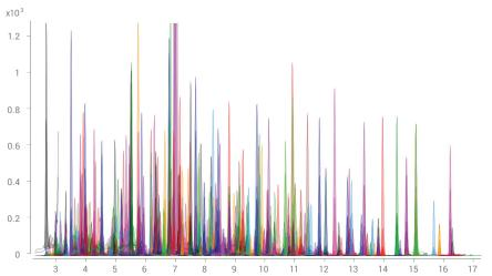
MRM signal response for 251 pesticides detected in black tea extract at 5 ng/g, which corresponds to  $\frac{1}{2}$  MRL or 1 ng/mL. The innovations within the Ultivo are critical for rendering sensitive detection.
