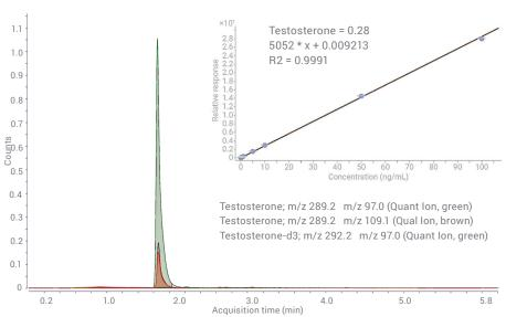
Overlaid MRM chromatograms showing elution of testosterone (500 pg/mL) and its d3-analog (internal standard; 25 ng/mL); calibration curve using a 1/x weighting factor.
