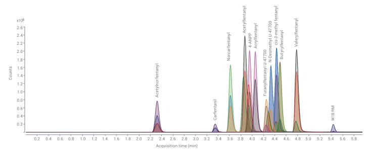
Composite MRM chromatograms of synthetic fentanyl compounds acquired in under 6-minutes on the Ultivo LC/TQ system.
