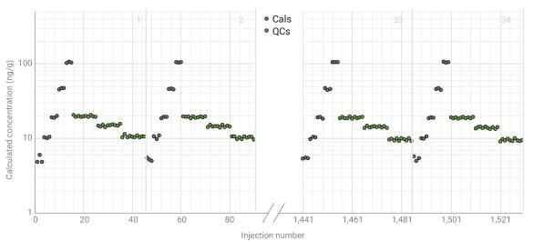
Experimental design for quantitation repeatability. Calculated concentrations for thiabenzadole are plotted for sample groups 1-2 (first 90 injections), and 3-4 (last 90 injections).
