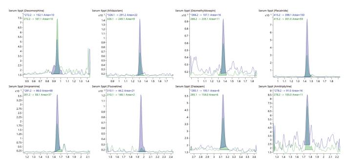
Extracted MRM chromatograms for the drug panel tested at 5.0 ppt.
