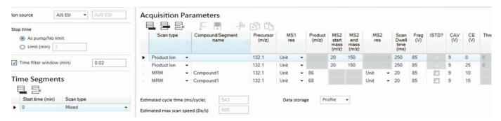
Acquisition parameter table showing low and high collision energy product ion and MRM scans for a mixed-mode acquisition for amino acid analysis where an analytical standard for hydroxyproline was not available.
