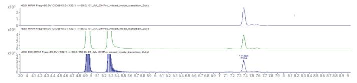
Low and high collision energy product ion and MRM scan for a mixed-mode acquisition showing isobars (leucine and isoleucine), as well as an MRM for an 'unknown' analyte (hydroxyproline).
