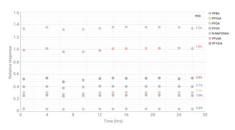
Uncorrected (without use of internal standards) relative area responses for 7 PFASs in 11-CCV samples over 26 hours.
