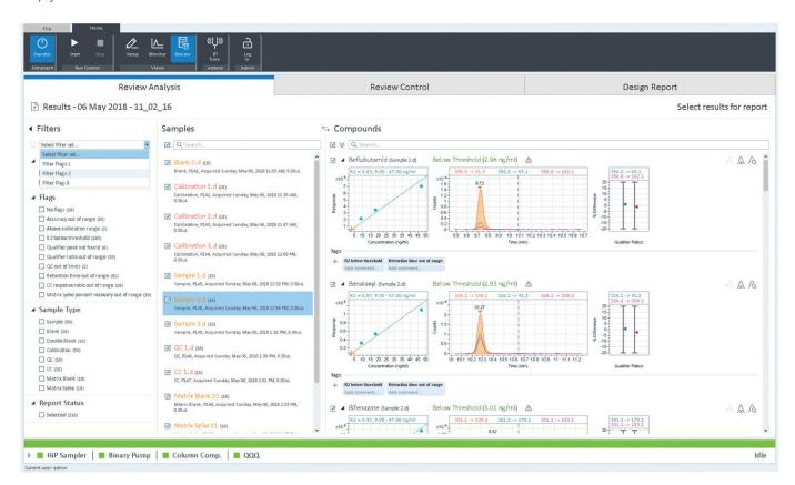
Easy and intuitive: Switch between "by sample" or "by compound" views with one click, and accelerate data review by applying individual flags or admin-defined filters.
