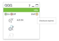
Early Maintenance Feedback (EMF) feature allows labs to plan for maintenance downtime instead of reacting when the instrument loses sensitivity or exhibits poor performance. It monitors the usage of specific components in the system and provides feedback when the user-selectable limits have been exceeded. The visual feedback in the user interface provides an indication that maintenance procedures should be scheduled. This leads to lower cost of ownership while increasing productivity.
