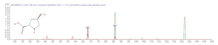
Low and high collision energy product ion scan for putative analyte 'hydroxyproline', showing the mechanistic decomposition for hydroxyproline (a first loss of carboxylic acid—[M-CO,H,] 46 Da, followed by a loss of water—[M-H,0] 18 Da).
