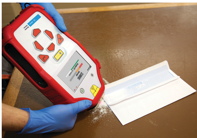
Figure 2. Line-of-sight surface scan mode.
