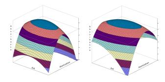
The Surface Response Methodology tool in the software uses chemometrics to automatically optimize the ash and atomize temperatures. Shown here is the plot for the standard reference material (left) and the spiked sample (right).
