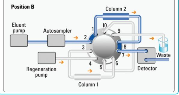
Figure 2. Alternating Column Regeneration valve configuration
