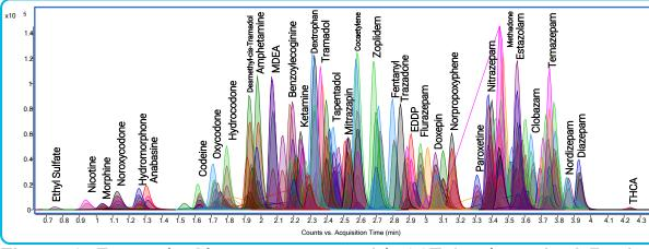
Figure 1. Example Chromatogram with 117 Analytes in 4.5 min
