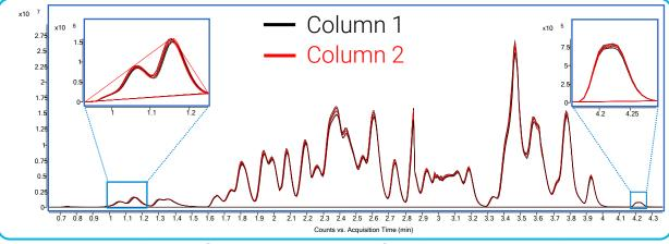
Figure 4. Overlays of 10 TIC traces of Column 1 vs. Column 2 Columns Comparison Test
