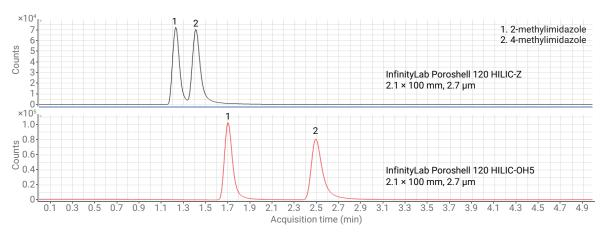
Figure 2. A comparison of the retention of 4-methylimidazole and 2-methylimidazole on an InfinityLab Poroshell 120 HILIC-Z and an InfinityLab Poroshell 120 HILIC-OH5 column with the same mobile phase.
