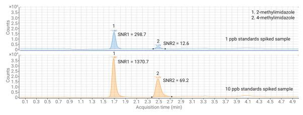
Figure 3. Chromatograms for 1 and 10 ppb standard spiked samples separated on an InfinityLab Poroshell 120 HILIC-OH5 column.
