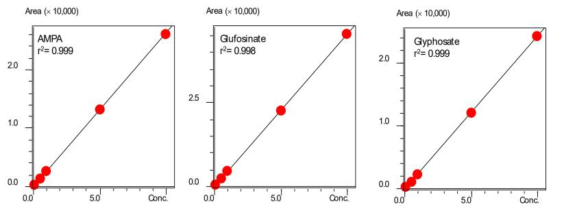
Figure 2 Calibration Curves of AMPA, Glufosinate and Glyphosate  $(0.1 \sim 100 \mu g/L)$
