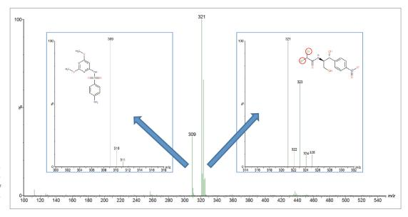
Example showing a negative ion mass spectrum, demonstrating the isotopic patterns of two compounds using the ACQUITY QDa Detector.
