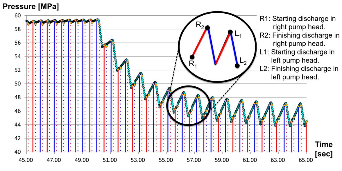
Fig. 5 Pressure transition when air bubbles are trapped in left pump head (Flow rate: 1mL/min, Pressure: 60MPa, Solvent: Water, Amount of air bubble: 5uL)
