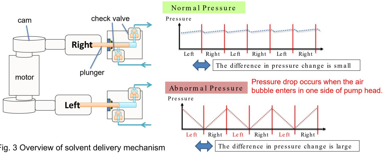
Fig. 3 Overview of solvent delivery mechanism
