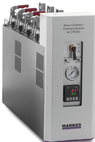
Figure 2. Markes \mu -CTE instrument: four-chamber model.
