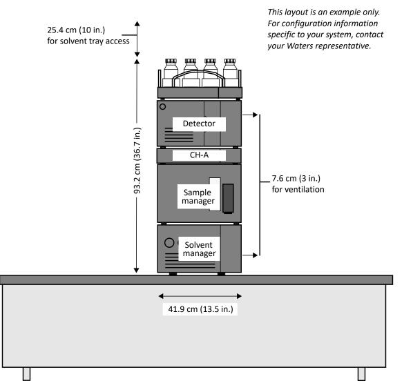
Figure 2 – One-stack configuration (example, front view)
