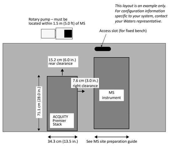
Figure 4 – Example configuration with MS (top view)
