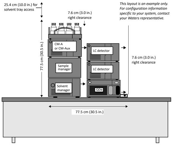
Figure 3 – Two-stack configuration (example, front view)
