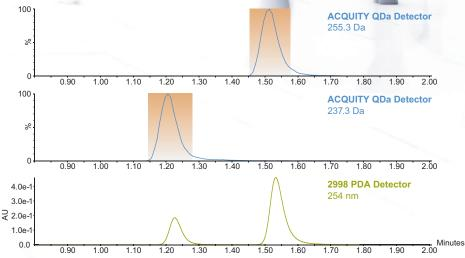
Fraction triggering by molecular mass, using the ACQUITY QDa Detector, allows selective isolation of each of the 2 components from this mixture separated using the Waters AutoPurification HPLC System.
