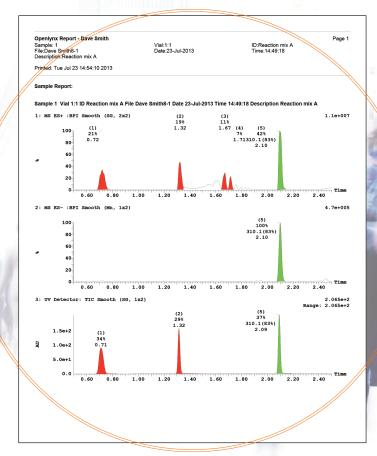
Typical open access report for a medicinal chemist using the ACQUITY UPLC System. The highlighted area shows how the ACQUITY QDa Detector confirms that the required product (310 Da) has been successfully synthesized while the purity is determined from the ACQUITY UPLC PDA Detector.
