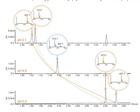
Manipulation of chromatographic mobile phases can produce substantial and useful alterations of separation selectivity. As applied to this mixture of Ziprasidone and USP designated related substances separated with the ACQUITY UPLC H-Class System, the orthogonal selective detection available with the ACQUITY QDa Detector permits the identification of coeluting species. With changes in mobile phase, individual analytes can be tracked through changes in relative retention.
