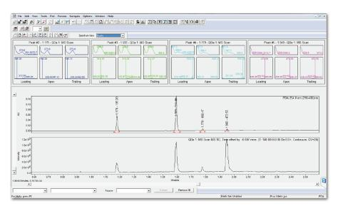
Confirm identities and highlight co-elutions in one workflow with the new Mass Analysis window in Empower 3 FR2. Chromatograms are annotated with both analyte mass and absorbance maximum, along with retention time, while the UV and mass spectra for each chromatographic peak are displayed together.
