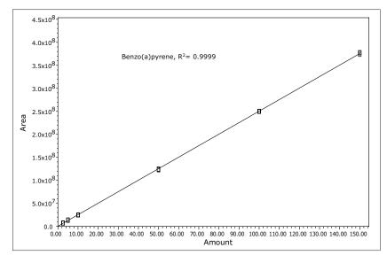
Figure 5. Calibration curve for benzo(a)pyrene (2.5 to 150.0 μg/L).
