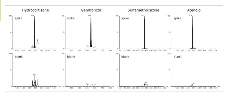
Figure 4. MRM chromatograms for example compounds that demonstrate blank responses in the extracted reagent water. The chromatograms in the top row demonstrate the expected response for the example compounds at the 0.1 ppt level (post-spiked into extracted reagent water). The bottom row shows the response in the blank extract of the reagent water.
