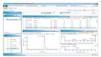
Figure 4. At 20.21 mins minor PFOS J (3mPFOS) isomer HDMS<sup>E</sup> fragmentation spectra that are ion mobility resolved from co-eluting PFOS isomer C.
