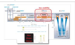
Figure 1. A schematic representation of the SYNAPT G2-S HDMS system and illustration of the mechanism of travelling wave ion mobility separations.
