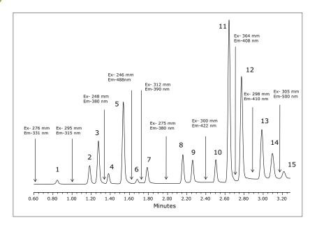
Figure 2. Separation of PAH analytes (0.1 mg/L) using timed programmed wavelength changes as indicated by arrows. PAH analytes are identified as follows:
