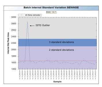
Figure 4. D4  $\beta$ -estradiol peak area plotted over a batch of samples.
