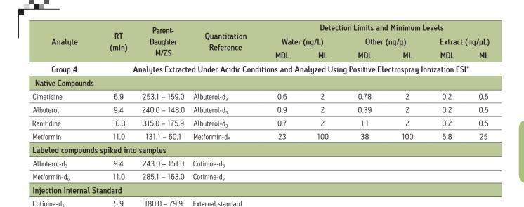
Group 4: Basic extraction positive electrospray ionization (ESI\*) compound retention times (RTs), parent-daughter transitions, quantitation references, method detection limits, and minimum levels of quantitation.
