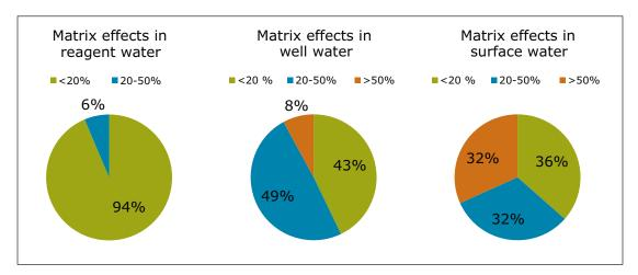
Figure 6. Pie charts showing the level of the matrix effects on the different PPCPs in three different water sample types. Low matrix effect (<20%) is shown in green; medium matrix effect (20% to 50%) is shaded blue; high matrix effect (>50%) is colored orange. The percentage of compounds showing the specified matrix effect are labeled on the pie segments.
