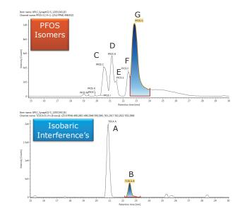
Figure 2. Accurate mass extracted ion chromatograms for the isobaric matrix interferences (Peaks A & B) and the PFOS isomers (Peaks C-G).
