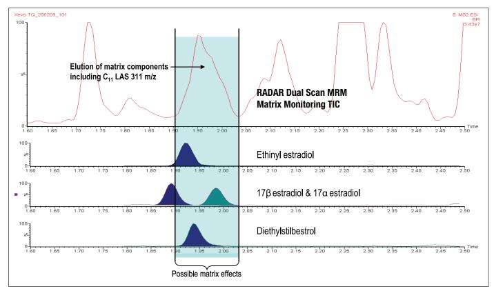
Figure 6. Expanded region of the same spiked sewage sample with some co-eluting of some matrix components including LAS, observed using RADAR Dual Scan-MRM matrix monitoring.
