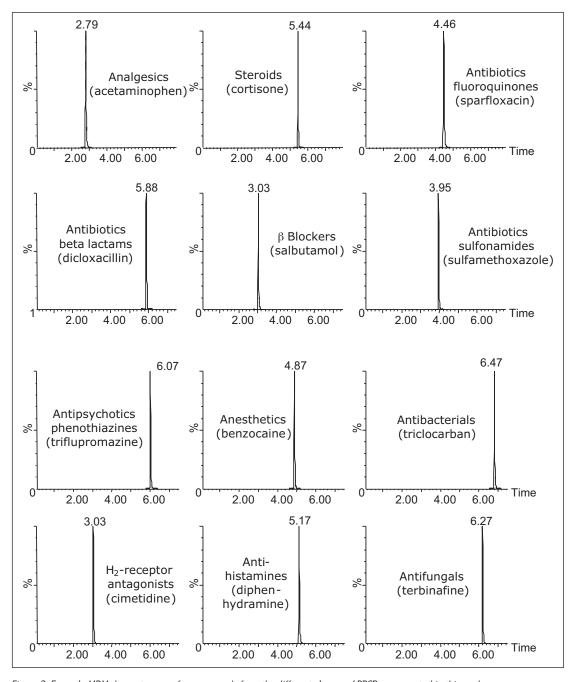
Figure 3. Example MRM chromatograms for compounds from the different classes of PPCPs represented in this work.
