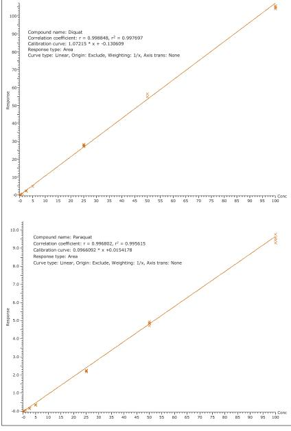
Figure 3A. Calibration curve for diquat from 50 ppt to 100 ppb.
