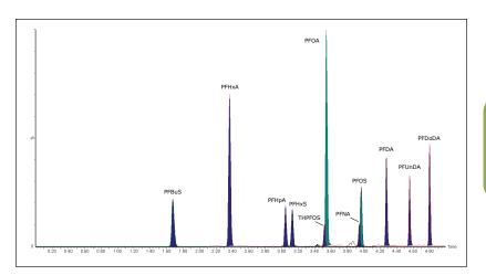
Figure 1. Overlaid MRM chromatograms of each target PFC (solvent standard; concentrations range between 1 pg/ $\mu$ L and 2 pg/ $\mu$ L).
