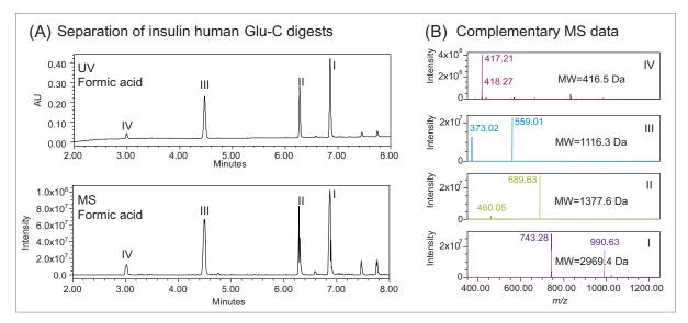
Figure 1. Separation of insulin human digest with orthogonal detection system using formic acid as mobile phase additive. Four peptide peaks were detected using (A) UV detection and MS detection by an ACQUITY QDa Mass Detector, with complementary MS spectra shown in (B).
