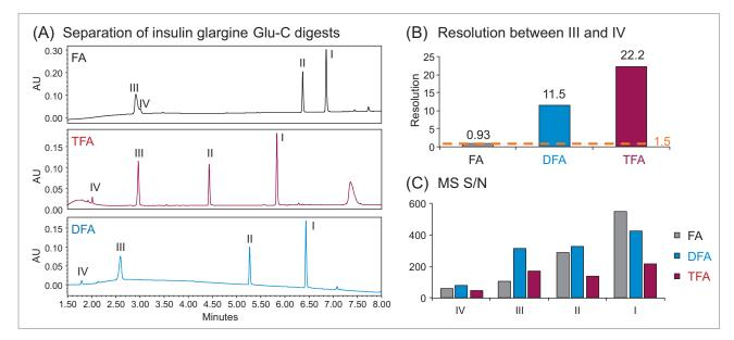
Figure 3. Comparison of different mobile phase additives. (A) Separation of insulin glargine digests using formic acid, TFA and DFA as mobile phase additive while keeping the gradient slope unchanged. (B) Bar plot of chromatographic resolution between the critical pair (Peak III and IV). Resolution using both DFA and TFA are above the 1.5 threshold. (C) MS signal to noise ratio (S/N) comparison for the four peaks.
