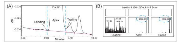
Figure 5. Mass Analysis assisted purity assessment of intact insulin. (A) separation of intact insulin. Blue dash lines indicate the cut-off of leading, apex, and trailing edge for the spectra displayed in (B) the Mass Analysis window in Empower. The apex and trailing window showed almost identical MS spectra, suggesting the main peak is relatively pure.
