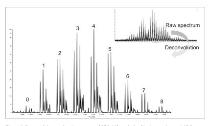
Figure 5. Raw and deconvoluted spectrum of SEC-MS analysis of Lysine conjugated ADC, Kadcyla (trastuzumab Entansine (T-DM1),) without deglycosylation. The number on top of the deconvoluted spectrum peaks represents the detected number of drugs that are conjugated to the protein Trastuzumab in the intact level. The calculated average DAR is 3.56, vs. the theoretical DAR of 3.50 [11].
