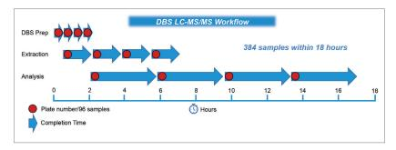
Figure 2. Analytical workflow for the analysis of DBS samples using Oasis MAX µElution SPE and UPLC-MS/MS analysis.
