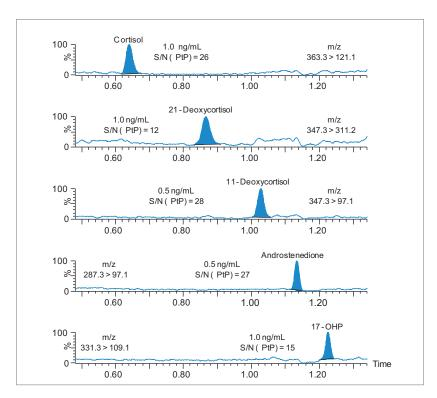
Figure 3. LLOQ chromatograms for cortisol, 21-deoxycortisol, 11-deoxycortisol, and 17-OHP in DBS samples.
