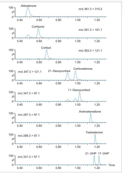
Figure 1. Chromatographic selectivity of the CORTECS™ C<sub>18</sub> 2.7 µm Column for the separation of cortisol, 11-deoxycortisol, 21-deoxycortisol, androstenedione, and 17-OHP from other endogenous steroid hormones.
