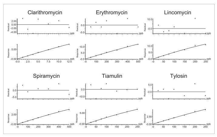
Figure 3. Typical calibration and residuals graphs for a selection of the macrolides.
