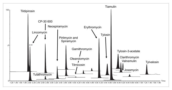
Figure 2. Chromatogram of a matrix-matched standard at the different MRLs showing all 18 macrolide antibiotics.
