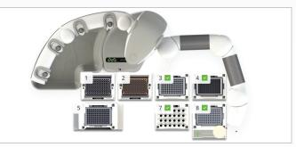
Andrew+ Domino configuration for the automated QC GlycoWorks RapiFluor-MS protocol. Domino/Device positions on the Andrew+ working deck: (1, 2) Tip Insertion Systems, (3) Storage Plate Domino, (4) Deep-Well Plate Domino, (5) Microplate Vacuum+, (6) Microtube Domino, (7) 96-PCR Peltier+.
