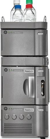
The ACQUITY PREMIER Solution significantly reduces analyte/surface interaction of sensitive compounds for improved chromatographic performance in RPLC/MS-based separations.
