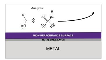
Figure 1. A MaxPeak High Performance Surface as utilized in the ACQUITY Premier Solution to impede electron rich analytes from interacting with metallic hardware.
